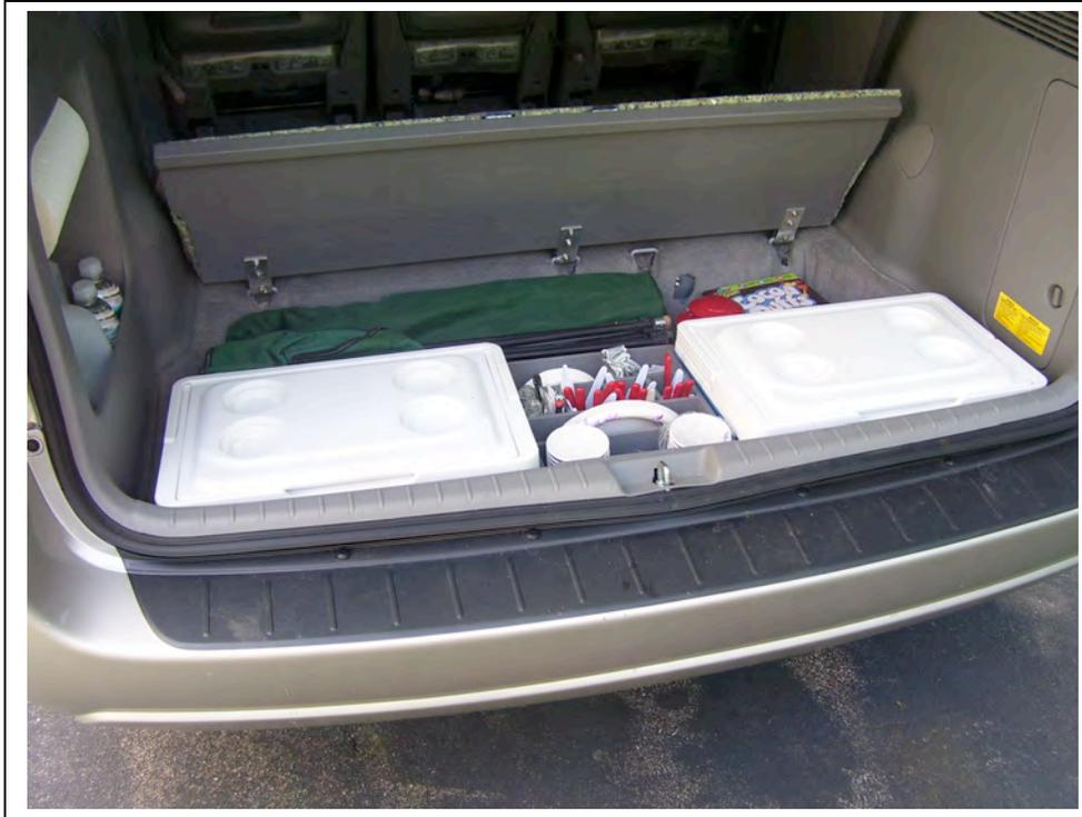
Normally, the third row seats fold into the rear well. By removing these seats and covering the top of the well with a plywood lid, a large amount of storage (8 cubic feet) is made available while 5 people can still sit comfortably in the van. As shown in the picture, two coolers with flat tops (26 quart size) fit perfectly into the back part of the well. One cooler functions as a refrigerator while the other is used to store baked and packaged goods.
