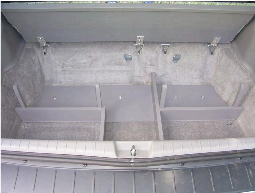
One of the goals of this project was to install the storage area framing and the lid over the well and attach them to the car without drilling holes or modifying the Sienna minivan in any way.
