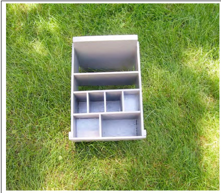
The plans also show the utensil organizer's construction: the sides are built of 3/8 inch plywood while the dividers are built of 1/4 inch plywood. They are all glued together and to the sides. The exact configuration is, of course, the designer's choice.
